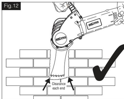
When using the Mortar Plunge blades, the cut should have enough clearance on each end (shown in fig:12), to ensure that no hammering of the blade ends occurs (as shown in Fig.13).
