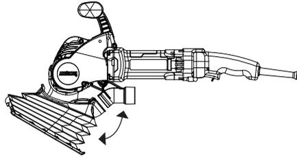
3. Pinch and fold the front tabs of Dust Boot and press underneath the guard rail.
