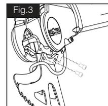
**NOTE: Blades are a wearing part. In normal operation, blade life may vary with the hardness of materials cut.**
