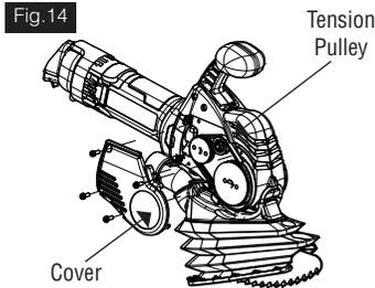
During belt tensioning or replacement a visual inspection of the pulleys should be completed, as they will wear due to excessive belt slip. Replacement may be required if the V profile grooves on the pulleys appear worn or damaged. To replace either pulley contact your ARBORTECH authorised service centre.
