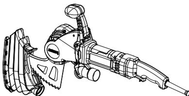
2. Pivot the Dust Boot until it engages with the dust extraction fitting and achieves a seated overlap
